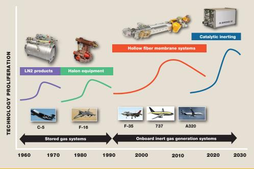
Bleeding engines to supply a conventional ASM-based inerting system can be particularly burdensome for aircraft powered by engines that have little or no
