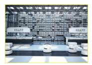
**OSR Shuttle™** – **KNAPP** shuttle systems form the heart of a modern warehouse. Solutions can be seamlessly integrated into the logistics system with customized software and ergonomic workstation solutions. Free moving open shuttles supply workstations and deliver totes, cartons or pallets. Driverless vehicles deliver up to 2800 lbs. **KNAPP** invented shuttle technology to realize centralized processing within the fulfillment center, with one single core technology.
