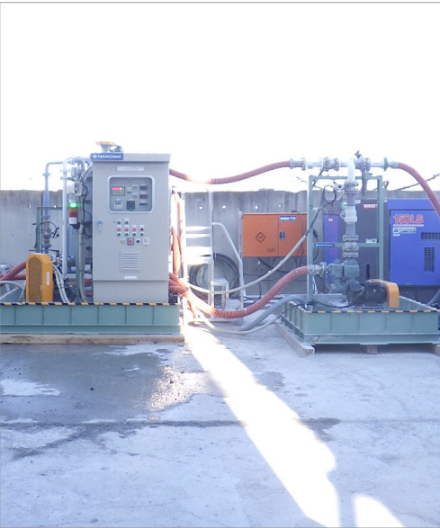
Taiheiyo's new CARBOCATCH system is being trialled on a public construction project in Japan. Lower carbon concrete is being produced by using waste materials that have absorbed CO 2 through the CARBOCATCH system. Read more on p74
